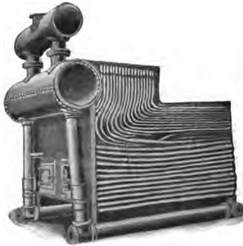
FIG. 14.—An Exploded Boiler. (A marine accident.)
